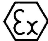
2 Equipment or Protective systems intended for use in Potentially Explosive Atmospheres - Directive 2014/34/EU
