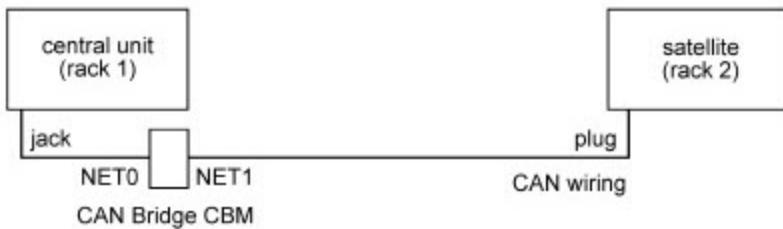
Figure 101 Connection CAN-Bridge CBM
