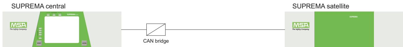
Figure 99 System with one satellite and CAN bridge
