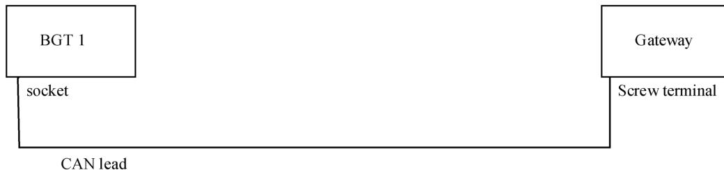
Figure 138 Connection SUPREMA Gateway Can/ Profibus DP
